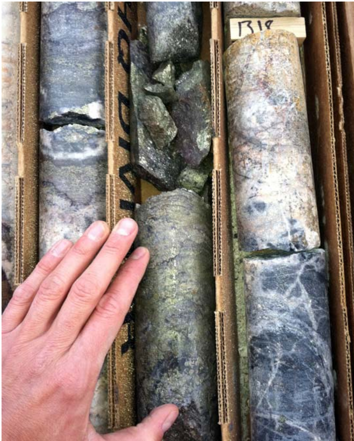
Above: Chalcophyrite-rich core sample.
