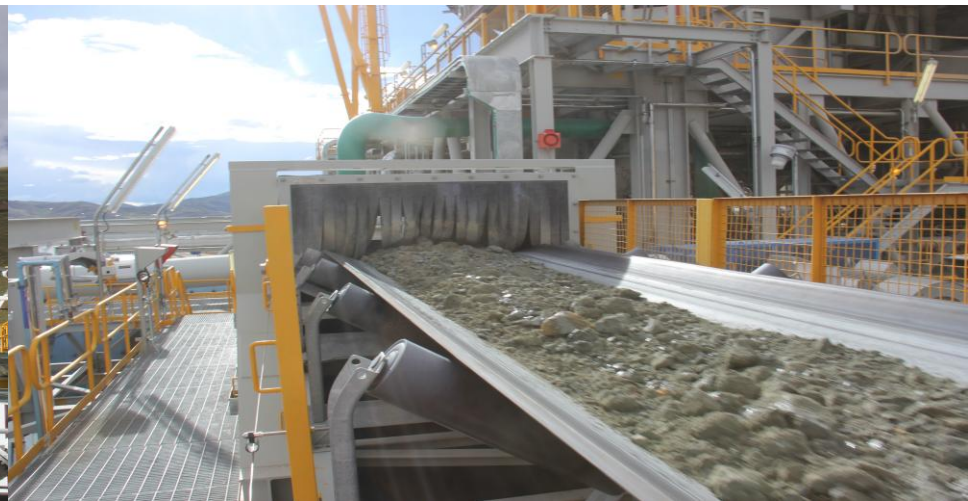
Crushed ore to be processed in Constancia mill
